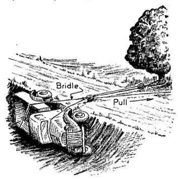
FIGURE 32.—Righting an overturned vehicle.
